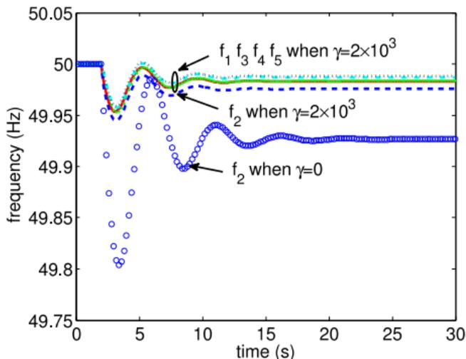
**Notes:** (i) Frequency deviations in area 2 are much smaller in the presence of the control scheme. (ii) The frequencies do not converge to the same value (iii) Voltage excursions in the DC grid are small (less than 1%).
