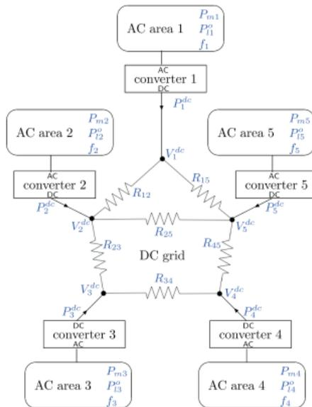
Frequencies ( $f_i$ ) and power produced by every area  $i$  ( $P_{m_i}$ ) are state variables.  $V_i^{dc}$  and  $P_i^{dc}$  are control variables.  $P_{i_i}^0$  is the power consumed by the load at the nominal frequency. If  $P_{i_i}^0$  increases (decreases),  $f_i$  drops if  $P_i^{dc}$  is kept at its reference value (which is determined by a market clearing mechanism).
